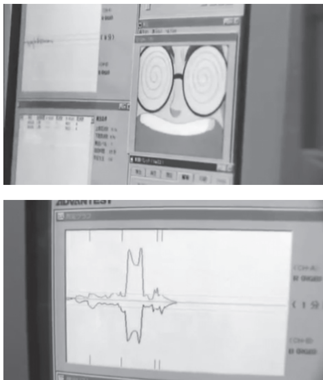
FIGURE 13.1. In one sequence in The Tube , personnel at TV Tokyo play clips of the notorious episode 38 of Pokémon , measuring the frequency of flicker for red and blue, which is mapped alongside the footage. The second image shows the measurements for the 12 Hz red–blue flicker scene, which jumps well outside the safety zone.
